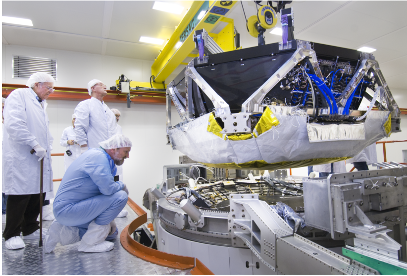
Figure 3.9: Pre-integration of the transition radiation detector (TRD) onto the AMS experiment. Image taken from Cern Document Server .
